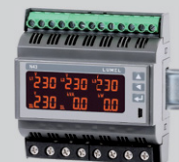
N43 - rail mounted 3-phase power network meter
