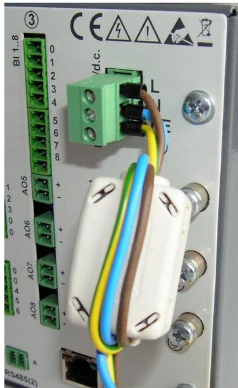
Fig. 1.1. Connection of the power supply filter.
