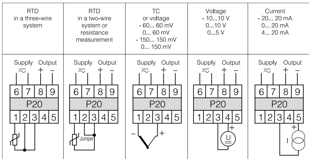
Coding of the P20 transducer input kind
