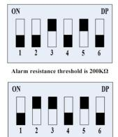
Alarm resistance threshold is  $600 \mathrm{K}\Omega$
