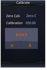
confirmation key again until the ADC value is stable (30 to 90 seconds), the pop screen shows "whether to calibrate!" Select Yes to calibrate the gas. Select No and return to the calibration interface. "The lower left corner shows "Ccalibration success!" after successful calibration.
