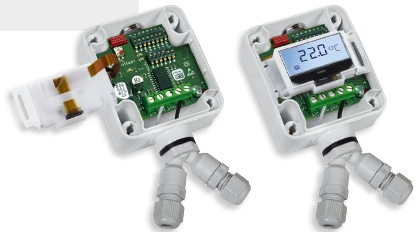
\* High-performance encapsulation against vibration, mechanical stress and humidity
