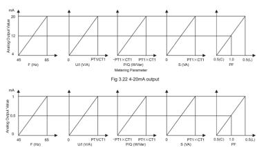
P/Q (W/Var) Metering Parameter Fig 3.23 0-1mA output
