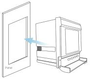
Fig 2.4 Put the meter into square hole
