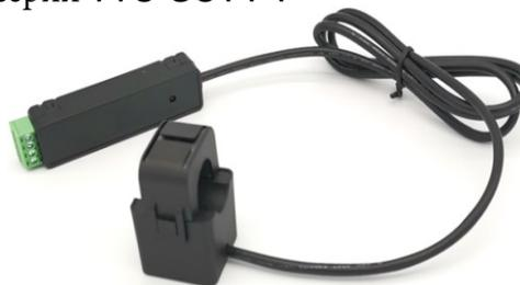
The current transmitter converts the AC current signal into a standard electrical signal, and drives and transmits it in a constant voltage or constant current mode; it has the advantages of high precision, small size, low power consumption, strong anti-interference ability, etc. It is especially suitable for motors and intelligent low voltage Intelligent monitoring system for load current such as power distribution cabinet and PLC automation.
