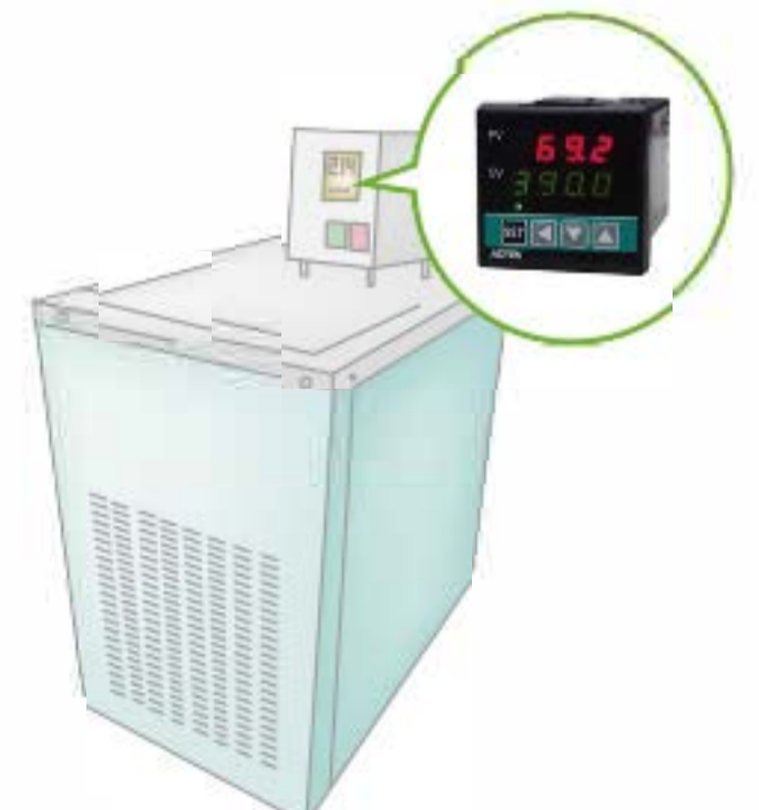
Temperature control in heated water tank
