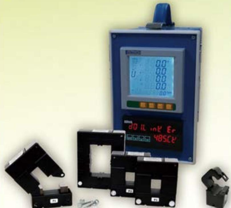
Combine the usage of DL1S and CPM-70 for recording the parameters. Chronological record the parameters (VAC, AAC, KW, KWH, PH, Hz, ...) and Power quality (1~31st Individual Harmonic, Un-balance, K Factor, Crest Factor, ...) in SD card of DL1S from multifunction power meter via a RS485 serial communication port, and providing ADPro software to convert the data into Excel spreadsheets (.xls) for analysis. Along with Split core CT such as US-CTS or US-CTA/ US-CTB for long-term Data-Logging.
