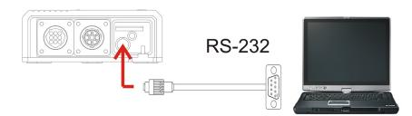
(See instruction manual to verify connections and maximum voltage of the device)
