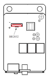
After changing the battery of the device must be set the time and an hour. To set the time should follow the instructions in Chapter 13. Setting the time of the analyzer
