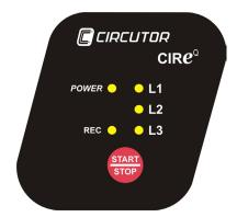
When you wish to stop the recording process, hold *START/STOP* during 3 seconds to stop and end the recording.
