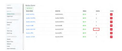
To view the Alarm click on the Device Name, and select the 'Alarms' tab. The alarm page displays the alarm conditions (max and min) as well as the current value of the parameter, the status of the alarm (on or off) and the action for this alarm (edit or delete). The alarms can also be viewed from the Alarm Logs which will be discussed later in the manual.
