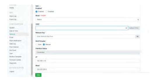
By default the WIFI mode is set for Access Point Mode, where the AcuLink 810 acts as a wireless bridge allowing other wireless devices to connect.
