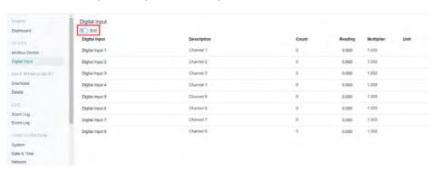
Enter in a Description and the units the pulses will be representing. A multiplier can be applied to the count if necessary. Users can also input a starting count value to the digital input channel.
