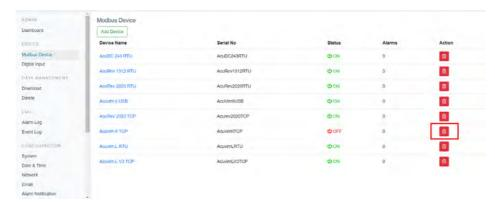
After selecting delete device, a message will appear asking the user to confirm the delete. Select 'Yes, Delete' to remove the device and all stored data from the AcuLink 810.
