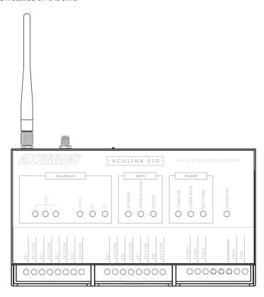
By default the AcuLink 810 has its WIFI mode set as AP (Access Point) mode, where the AcuLink 810 acts as a wireless access point allowing other wireless devices to connect and access the gateway.
