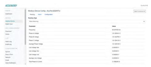
The Device data can be viewed on the 'Reading' tab.
