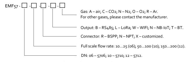
Note: 1. For CO2 and N2O, the full-scale flow rate is 80% of air.
